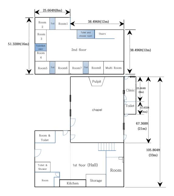
Chapel size: 67.368ft(21m)\*38.496ft(12m)=2,712ft<sup>2</sup>(252m<sup>2</sup>) 1st floor size:2,928ft<sup>2</sup>(272m<sup>2</sup>) 2nd floor size:2,928ft<sup>2</sup>(272m<sup>2</sup>)
